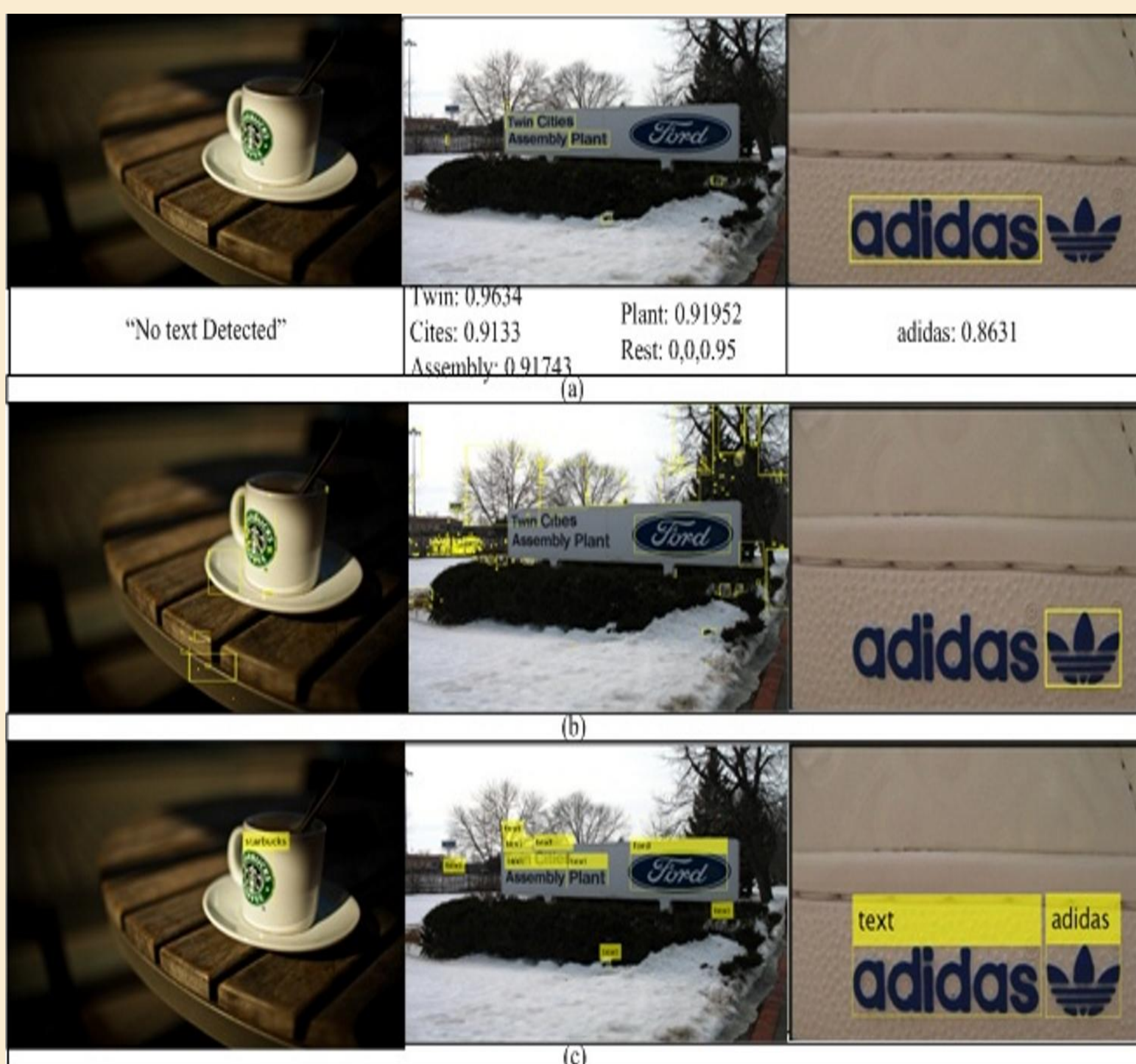
Assessment of the proposed method using three different types of logo images. (a) Word formation and subsequent OCR application. (b) Logo candidate generation. (c) Final Output Images.
