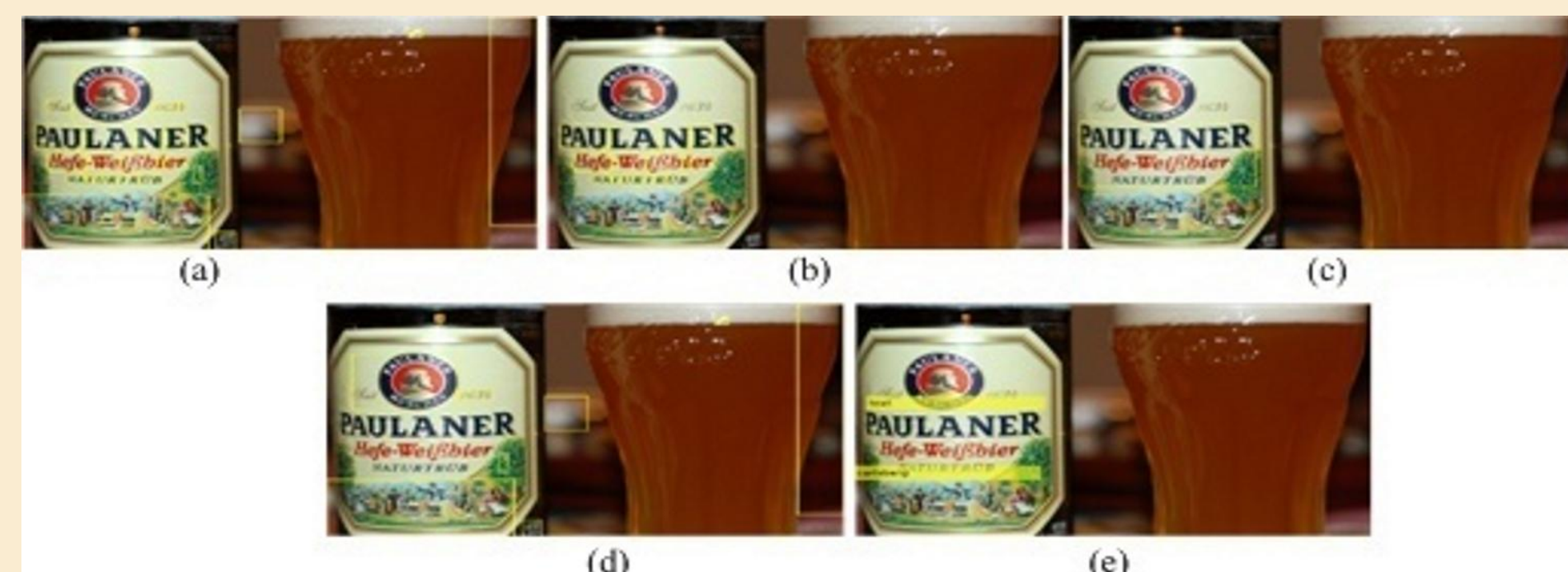
(a) Character proposals. (b) Detected characters. (c) Detected text region. (d) Logo region proposals. (e) Output image. Text lines (noise), placed too close to the logo, form part of the logo and our logo recognition mechanism fails. The problem can be addressed by incorporating more training data with increased noise levels.
